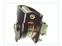
This Self Closing cap automatically protects the RJF TV square flange receptacle (MIL-DTL-38999 type), protecting your system from dust and water projection. A spring automatically closes the upper part of the cap when the RJF TV plug is removed from the receptacle.
