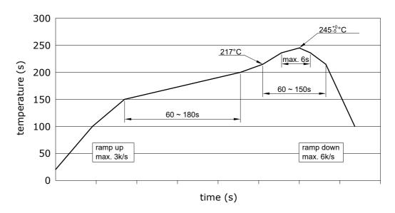
Figure 3. Recommended reflow oven temperature profile
