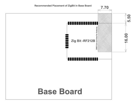
The ZigBit's location and orientation on the carrier board is illustrated in the above Mounting information drawing. The Recommended placements of ZigBit on Carrier Board needs to be accurately followed to ensure performance on the end application.
