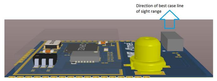
The Antenna in this module is designed to provide the best possible LoS range in the direction indicated in this illustration.
