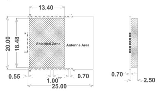
Figure 3-2. ATZB-RF-233-1-C Pinout
