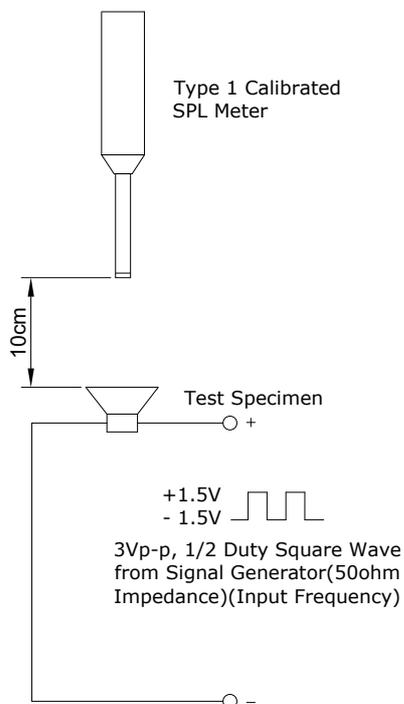
**Figure 2. Test Setup**
