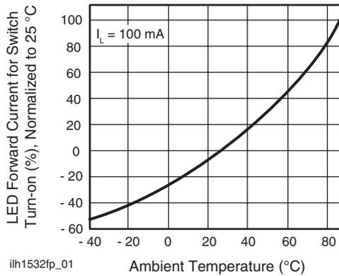
Fig. 1 - LED Current for Switch Turn-on vs. Temperature
