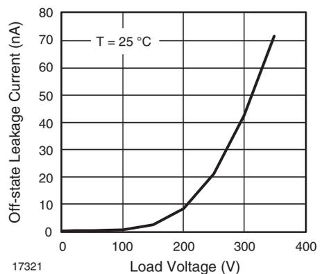
Fig. 6 - Leakage Current vs. Applied Voltage
