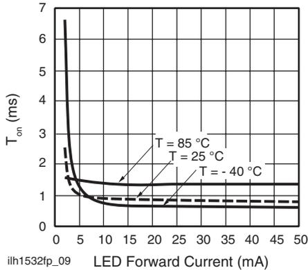
Fig. 9 - Turn-on Time vs. LED Current
