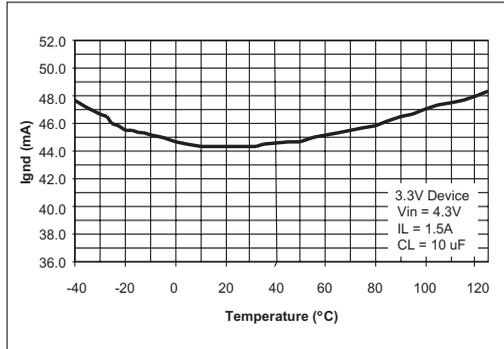
**Figure 13. Ground Current vs Temperature at  $I_{LOAD}=1.5A$**
