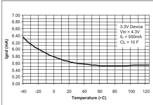
**Figure 11. Ground Current vs Temperature at  $I_{LOAD}=500mA$**
