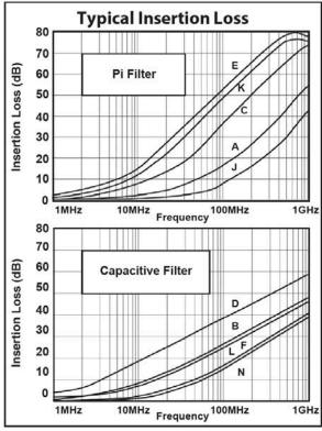
Insertion loss measured per MIL-STD-220, no load, 50ohm source and load.
