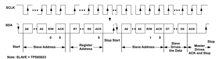
Figure 34. Serial i/f READ from TPS65023, TPS65023B: Protocol B
