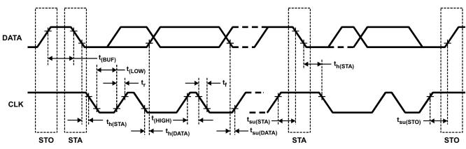
Figure 35. Serial i/f Timing Diagram
