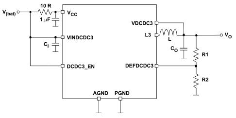
Figure 36. External Resistor Divider
