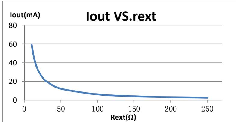
Diagram 1. Relation Curve between SM2082D Output Current and r<sub>ext</sub>
