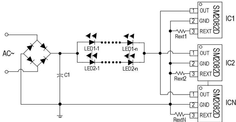
Diagram 6. Circuit Schematic Diagram of Parallel Application
