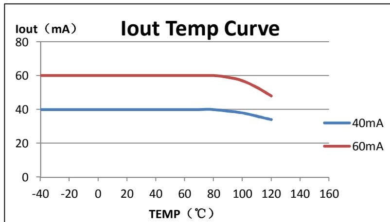
Diagram 3. SM2082D Output Current Temperature Characteristic
