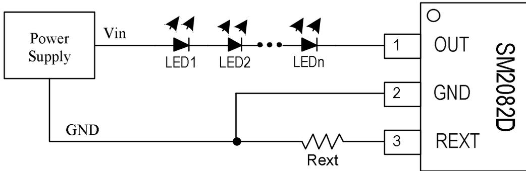
Diagram 4. SM2082D Application Circuit Schematic Diagram
