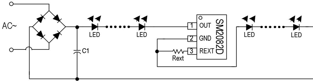
Diagram 7. SM2082D Cascaded in LED Tube Lamp
