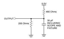
Figure 1: AC Output Loading
