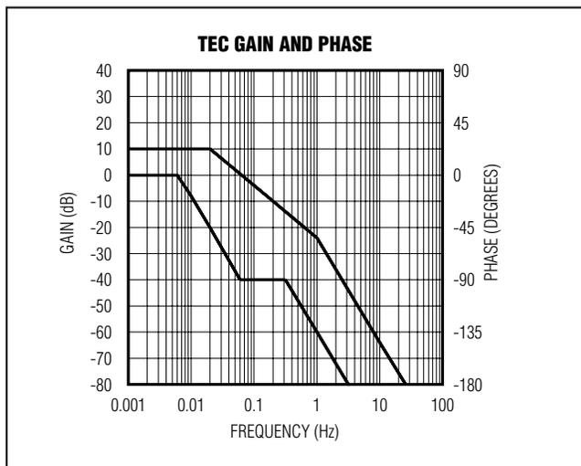
Figure 6. Bode Plot of a Generic TEC Module
