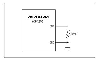
Figure 2. Setting the Current Limit
