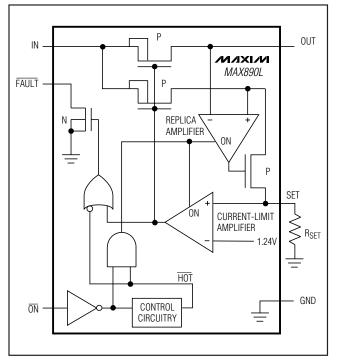
Figure 1. Functional Diagram
