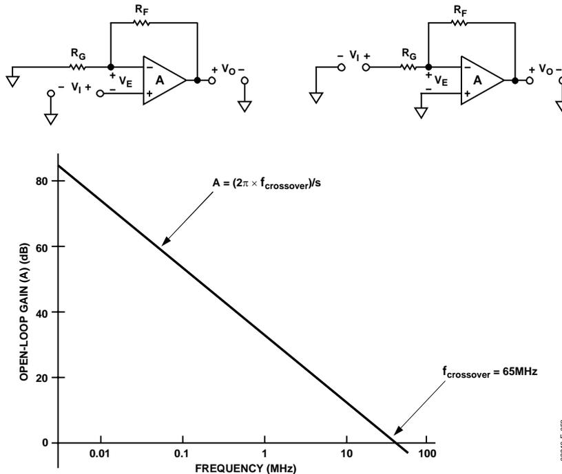
Figure 53. Open-Loop Gain vs. Frequency and Basic Connections
