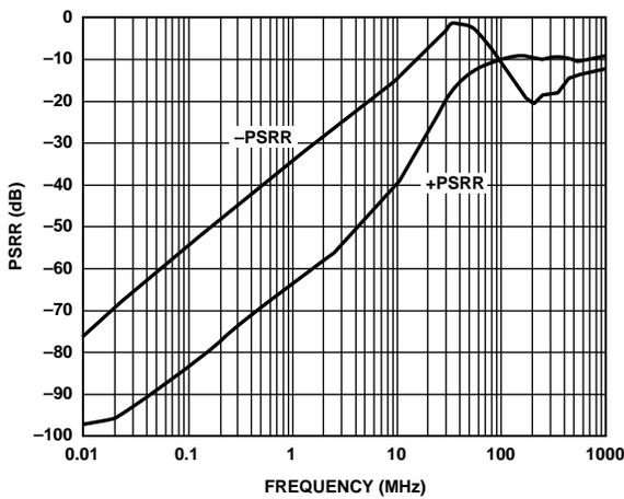
Figure 36. PSRR vs. Frequency (See Figure 48 and Figure 50)
