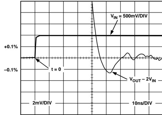
Figure 31. 0.1% Short-Term Settling Time (See Figure 49)
