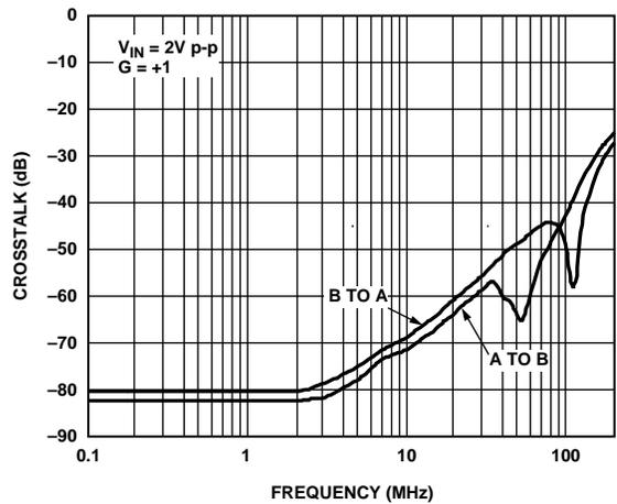
Figure 39. Crosstalk vs. Frequency (See Figure 51)
