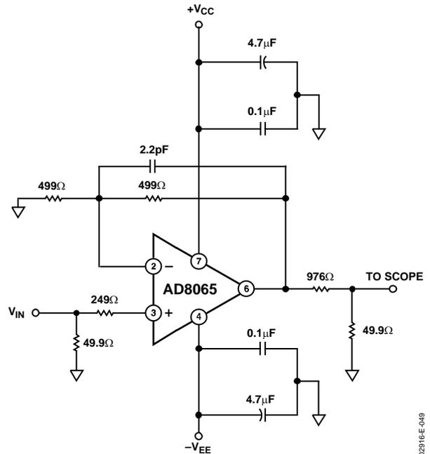
Figure 49. Settling Time
