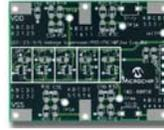
This blank PCB allows quick evaluation of Voltage Supervisors and Voltage Detectors in the SOT-23-5 and SOT-23-6 packages. This PCB supports many Microchip devices, including the non-volatile Digital Potentiometer and PIC10F2XX devices.
