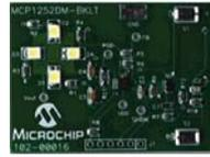
Demonstrates the use of a charge pump device in an LED application and acts as a platform to evaluate the MCP1252 device in general. Light intensity is controlled uniformly through the use of ballast resistors.
