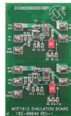
Features a 1A 1.4 MHz synchronous buck regulator in two buck converter applications. The applications use the 8-lead MSOP and 8-lead DFN packages respectively. Selectable output voltages and a shutdown terminal are available on each converter.
