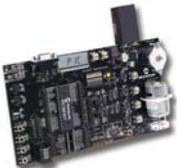
Learn how to use PIC® MCUs to enhance or replace a mechanical design. This demo kit takes a hands-on approach to learning about mechatronics. Jumper wires are provided in the kit and allow the user to experiment by connecting the PIC MCU to various components on the board. These components include sensors, LEDs, human input devices and motor drivers. The board comes with nine example projects and includes firmware, connection diagrams and schematics.
