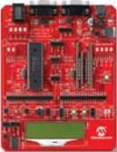
A development and evaluation tool to help create embedded applications using dsPIC30F DSCs. Sockets are provided for 28- and 40-pin devices in the motor control family and 18-, 28- and 40-pin devices in the general purpose and sensor family.
