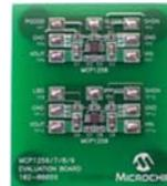
An evaluation and demonstration tool for the MCP1256/7/8/9 regulated 3.3V, low-ripple charge pumps with low-operating current Sleep mode or Bypass mode. The board is set-up to evaluate simple, stand-alone, DC-to-DC conversion. The two evaluation circuits provided, demonstrate the versatility of the MCP1256/7/8/9 family.
