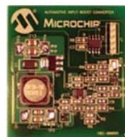
Demonstrates the MCP1630/V high-speed pulse width modulator used for automotive applications. When used with a microcontroller, the MCP1630/V devices control the power system duty cycle to provide regulated output voltage. The programmable PIC12F683 microcontroller is used to provide oscillator pulses at switching frequency of 500 kHz and set maximum duty cycle. The user may also modify or develop their own firmware routines to further evaluate the MCP1630/V devices in this application.
