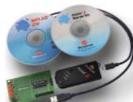
PICkit<sup>™</sup> 2 is small, easy-to-use starter kit that enables users to start writing code and programming with PIC<sup>®</sup> MCUs. Features full-speed USB support and firmware upgradeability in a low-cost tool. Includes a low pin-count demo board. Upgrade firmware for debugger function.
