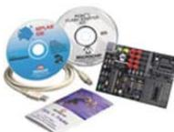
A low-cost starter development kit with an easy-to-use interface for programming Microchip's 8-/14-pin Flash PIC<sup>®</sup> MCUs. The kit includes everything needed to program, evaluate and develop applications. Seven tutorials with all source code files are furnished.
