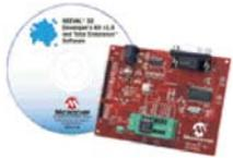
An evaluation and programming system supporting all Microchip Serial EEPROMs including future devices. Using a ZIF socket, standard DIP sockets are directly supported. The SEEVAL 32 gives the designer the ability
