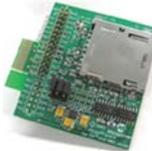
This PICtail daughter board interfaces with newer development boards that offer the PICtail and PICtail Plus connector interface; such as the PICDEM™ FS USB development board. This board also interfaces with the Explorer 16 Development Board via the PICtail Plus connector.
