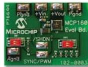
For both battery-powered and distributed-power applications. Operates over a 2.7V to 5.5V input range while delivering 500 mA of output current.
