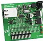
Provides a cost-effective method of evaluating and developing Ethernet-control applications. This board is populated with a 28-pin Ethernet controller, which interfaces to the RJ-45 female connector. Designed for flexibility, this board
