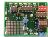
Provides a versatile selection of input channels and gains to evaluate device performance. Board supports multiple input signal sources. Two devices can be cascaded to produce gain to 1024 V/V.
