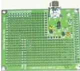
In combination with the PICDEM MSC1 Demo Board, this board serves as a demonstration and evaluation kit for designing high-resolution Delta Sigma Analog-to-Digital Converters using the PIC16C781/782.
