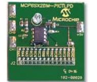
Opens possibilities to process other sensor signals. Increases the number of PIC® MCU I/O pins available for other purposes. Features a PNZ334 photo-diode, MCP6001U op amp and MCP6S22 and MCP6S92 Programmable Gain Amplifiers (PGA).
