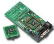
This low-cost demo board is used to evaluate the performance of High Pin Count (HPC) 8-bit PIC18F series microcontrollers. The board features a PIC18F8722 MCU, which is the superset of the entire 64- and 80-pin PIC18FXXX general purpose family. A daughter
