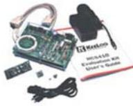
This kit demonstrates the capabilities of the code-hopping technology used in security systems such as garage door openers, auto keyless entry, etc. for secure access and/or authentication. It includes a main board and
