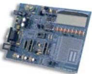
A demonstration and evaluation board for the 8-, 14- and 18-pin general purpose products with power-management features. It comes with two pre-programmed Flash-based MCUs, the PIC18F1320 and PIC16F627A, which both feature nanoWatt Technology.
