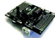
This board evaluates/demonstrates Microchip's MCP6S21/2/6/8 Programmable Gain Amplifier (PGA) family. Interface this board with the PICTail™ 1 Flash Starter Kit to demonstrate firmware integration between the PIC® MCU and PGA devices, while allowing modification and development of firmware for specific requirements.
