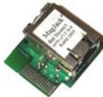
This board provides a cost-effective method of evaluating and developing Ethernet-control applications. Designed for flexibility, the board can be plugged into Microchip's Explorer 16 Development Board (DM240001). The board
