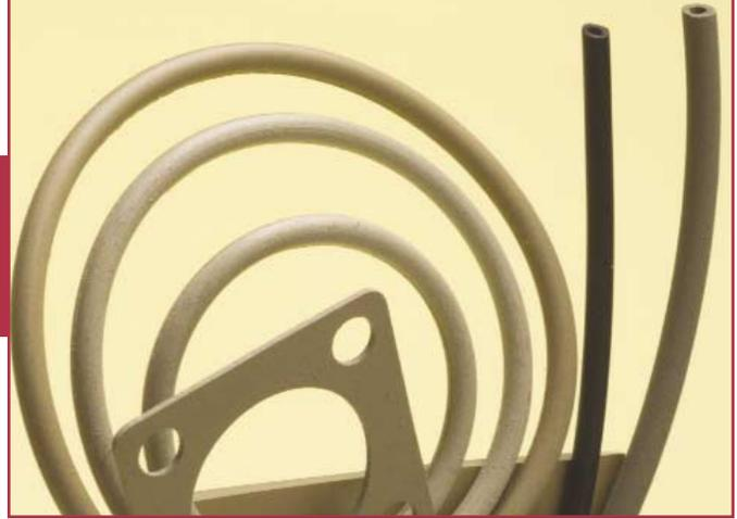
Spectrum Control's conductive elastomers are composed of silicon rubber using its heat resistant property. Unique features of conductive elastomers include water resistance and elimination of static electricity, which is different from general foam gaskets. It also acts as an absorber at high frequency showing 60dB shielding at 30MHz ~ 10GHz.
