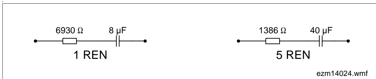
Figure 2-14 Typical Ringer Loads of 1 and 5 REN used in US
