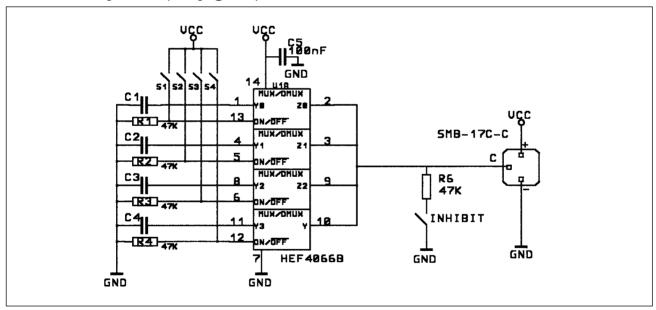
This typical application description is not limited to the typical components we have illustrated. Many other possibilities exist to select and switch the capacitors and/or the resistor.
