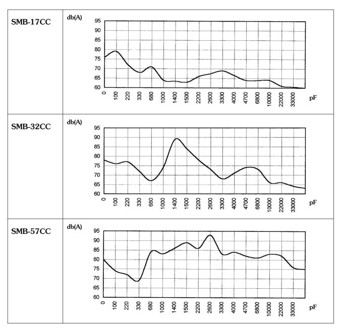
Measurements are made at 12 Vdc at 30 cm in free air at 21°C.
