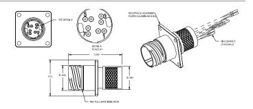
Jam Nut Receptacle Assembly, PC Tail Part Number 2102351
