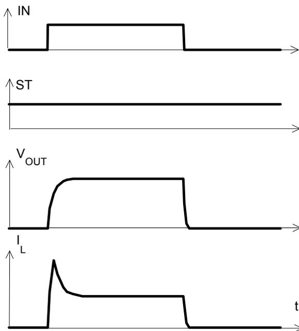
The initial peak current should be limited by the lamp and not by the initial short circuit current  $I_{L(SCp)} = 14 \text{ A}$  typ. of the device.
