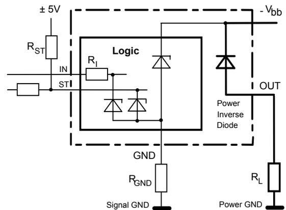
$R_{GND} = 150 \Omega$ ,  $R_1 = 3.5 \text{ k}\Omega \text{ typ.}$
