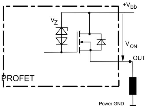
$V_{ON}$  clamped to  $V_{ON(CL)} = 47 \text{ V typ.}$
