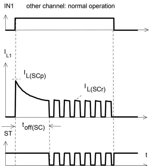
Heating up of the chip may require several milliseconds, depending on external conditions ( $t_{off(SC)}$  vs.  $T_{j,start}$  see page 12)
