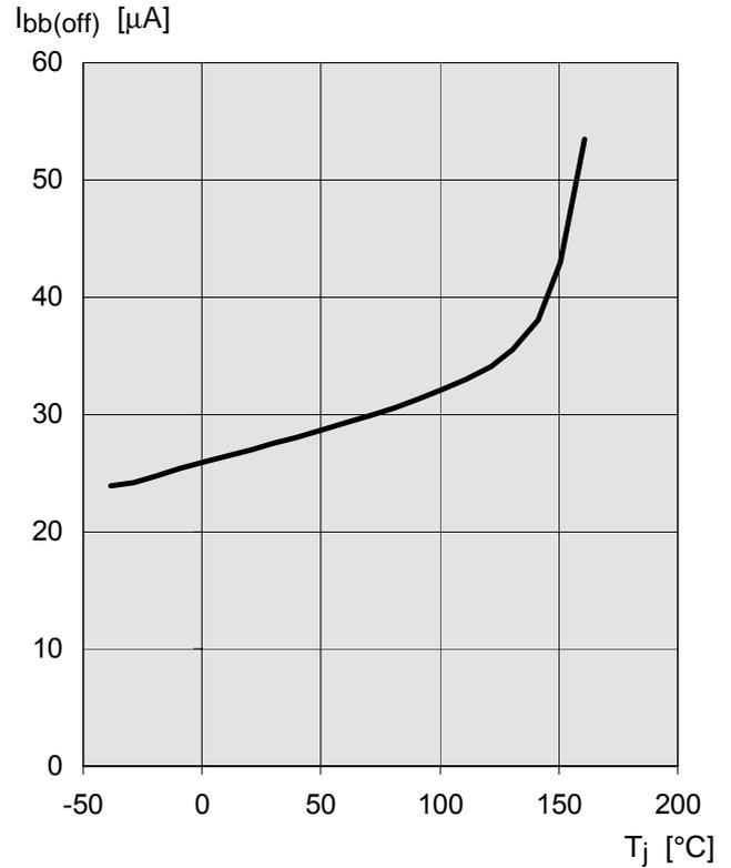
**Typ. open load detection current**
