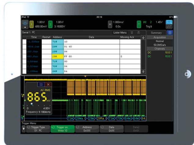
Figure 36: Tablet virtual front panel control.
