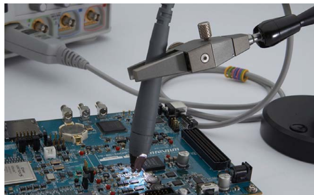
Figure 33: The N2750A InfiniiMode probe allows convenient measurement of differential, single-ended, and common mode signals with a single probe tip without reconnecting the probe to change the connection.
