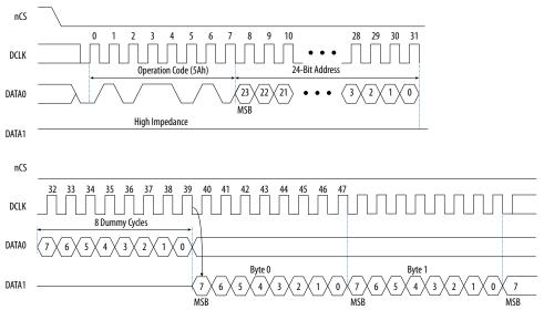
Initiate the Read SFDP operation by driving the nCS pin low and shifting the operations code followed by a 3-byte address into the DATAO pin. The 3-byte address content:
