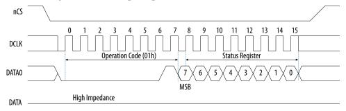
Immediately after the nCS signal drives high, the device initiates the self-timed write status cycle. The self-timed write status cycle usually takes 10 ms for all EPCQ-A devices and is guaranteed to be less than 15 ms. For details about  $t_{WS}$ , refer to the related information below. You must account for this delay to ensure that the status register is written with the desired block protect bits. Alternatively, you can check the
