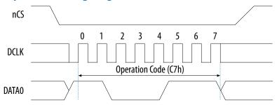
The device initiates a self-timed erase bulk cycle immediately after the nCS signal is driven high. For details about the self-timed erase bulk cycle time, refer to  $t_{EB}$  in the related information below.
