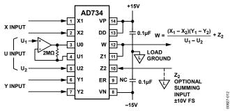
Figure 29. Three-Variable Multiplier/Divider Using Direct Denominator Control
