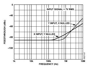
Figure 9. Feedthrough vs. Frequency
