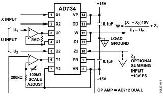
Figure 31. Two-Quadrant Divider with Fixed 10 V Scaling
