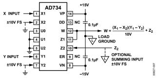
Figure 24. Basic Multiplier Circuit
