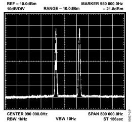
Figure 38. AD734 Third-Order Intermodulation Performance for  $f_1$  = 9.95 MHz,  $f_2$  = 10.05 MHz, and  $f_0$  = 9.00 MHz and for Signal Levels of  $f_1$  =  $f_2$  = 0 dBm and  $f_0$  = +24 dBm (All Displayed Signal Levels Are Attenuated 20 dB by the 10X Probe Used to Measure the Mixer's Output)
