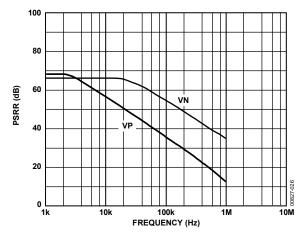
Figure 8. PSRR vs. Frequency
