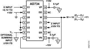
Figure 27. Standard (AD534) Divider Connection
