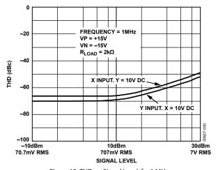
Figure 12. THD vs. Signal Level, f = 1 MHz
