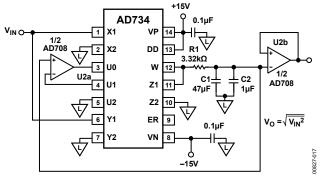
Figure 34. A Two-Chip, Wideband RMS-to-DC Converter
