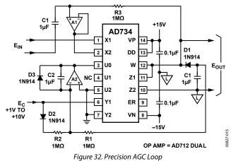
Diode D1 and C1 form a peak detector, which rectifies the output and causes the integrator to ramp positive. When the current in R1 balances the current in R2, the integrator output holds the denominator output at a constant value. This occurs when there
