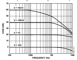
Figure 30. Three-Variable Multiplier/Divider Performance
