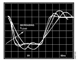
Figure 15. Pulse Response vs.  $C_{LOAD}$ ,  $C_{LOAD} = 0$  pF, 47 pF, 100 pF, 200 pF
