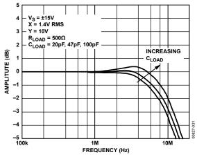
Figure 13. Gain vs. Frequency vs. CLOAD
