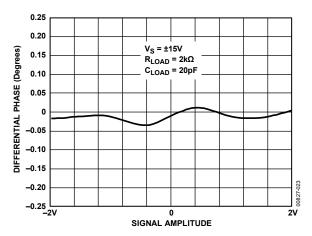
Figure 5. Differential Phase at 3.58 MHz and  $R_{LOAD} = 2 k\Omega$
