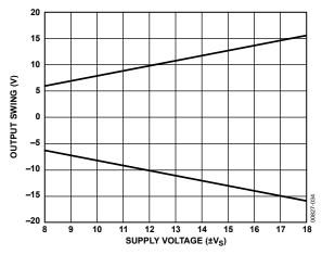
Figure 16. Output Swing vs. Supply Voltage
