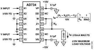
Figure 25. Conversion of Output to a Current
