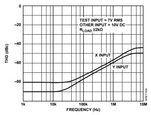
Figure 11. THD vs. Frequency, U = 10 V
