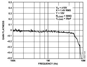
Figure 6. Gain Flatness, 300 kHz to 10 MHz,  $R_{LOAD} = 500 \Omega$
