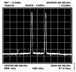
Figure 37. AD734 Third-Order Intermodulation Performance for  $f_1$  = 9.95 MHz,  $f_2$  = 10.05 MHz, and  $f_0$  = 9.00 MHz and for Signal Levels of  $f_1$  =  $f_2$  = 6 dBm and  $f_0$  = +24 dBm (All Displayed Signal Levels Are Attenuated 20 dB by the 10X Probe Used to Measure the Mixer's Output)
