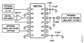
Figure 36. AD734 Mixer Test Circuit
