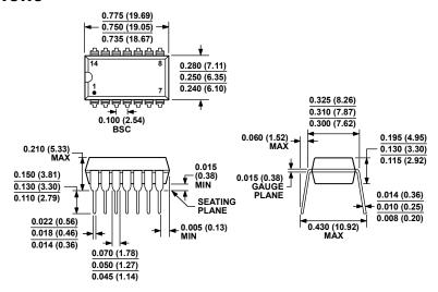
**COMPLIANT TO JEDEC STANDARDS MS-001** CONTROLLING DIMENSIONS ARE IN INCHES; MILLIMETER DIMENSIONS (IN PARENTHESES) ARE ROUNDED-OFF INCH EQUIVALENTS FOR REFERENCE ONLY AND ARE NOT APPROPRIATE FOR USE IN DESIGN. CORNER LEADS MAY BE CONFIGURED AS WHOLE OR HALF LEADS.
