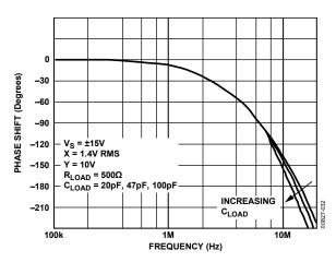
Figure 14. Phase vs. Frequency vs. CLOAD
