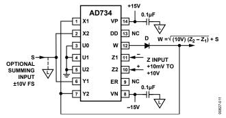
Figure 28. Connection for Square Rooting
