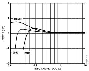
Figure 33. AGC Amplifier Output Error vs. Input Voltage
