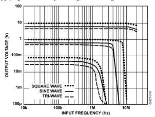
Figure 35. RMS-to-DC Converter Performance
