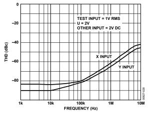
Figure 10. THD vs. Frequency, U = 2 V
