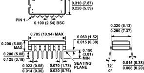
CONTROLLING DIMENSIONS ARE IN INCHES; MILLIMETER DIMENSIONS (IN PARENTHESES) ARE ROUNDED-OFF INCH EQUIVALENTS FOR REFERENCE ONLY AND ARE NOT APPROPRIATE FOR USE IN DESIGN.
