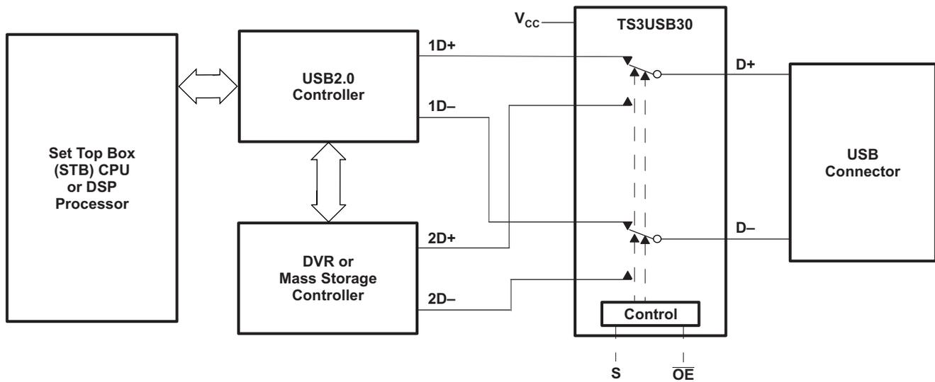
Figure 4. Application Diagram
