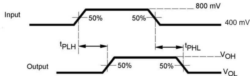
Figure 12. Propagation Delay
