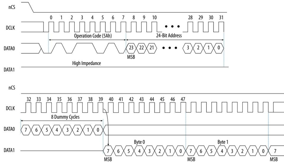
Initiate the Read SFDP operation by driving the nCS pin low and shifting the operations code followed by a 3-byte address into the DATA0 pin. The 3-byte address content:
