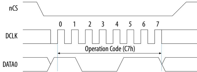
The device initiates a self-timed erase bulk cycle immediately after the  $nCS$  signal is driven high. For details about the self-timed erase bulk cycle time, refer to  $t_{EB}$  in the related information below.
