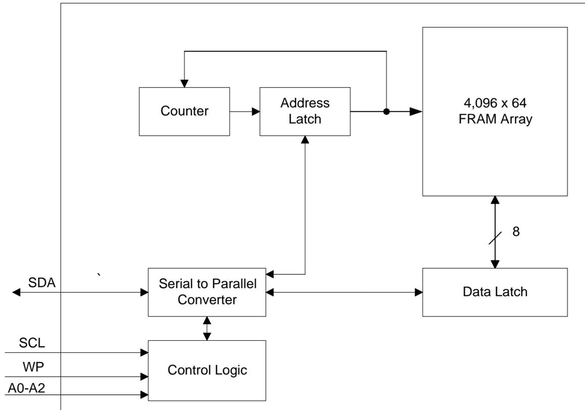
Figure 1. Block Diagram
