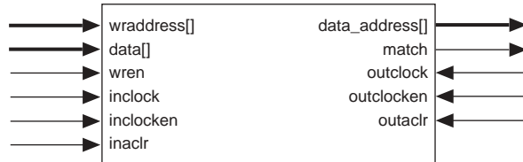
Figure 23. APEX 20KE CAM Block Diagram
