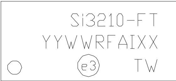
Figure 40. TSSOP Top Mark Diagram
