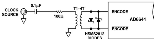
Figure 25. Crystal Clock Oscillator – Differential Encode
