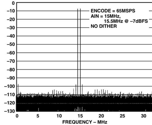
Figure 17. Two Tones at 15 MHz and 15.5 MHz
