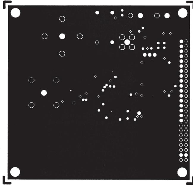
Figure 35. AD6644ST/PCB Ground Layer – Layers 2 and 5 (Negative)
