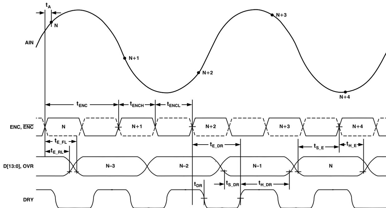
Figure 1. Timing Diagram
