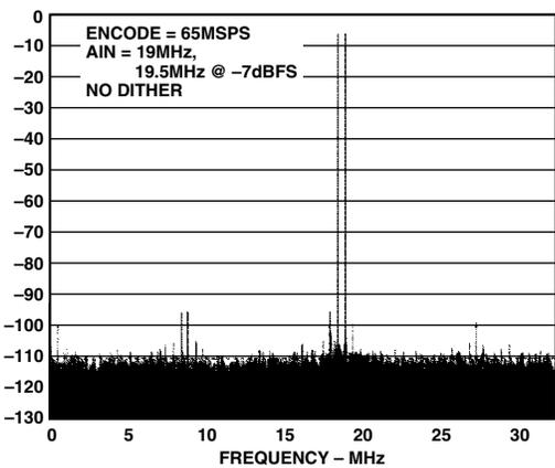
Figure 16. Two Tones at 19 MHz and 19.5 MHz
