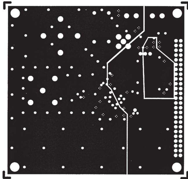
Figure 36. AD6644ST/PCB "Split" Power Layer – Layers 3 and 4 (Negative)
