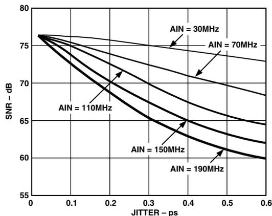
Figure 29. SNR vs. Jitter
