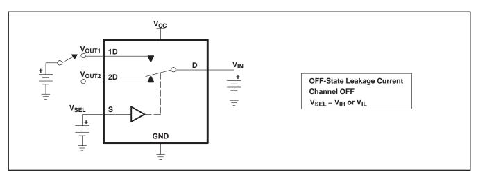
Figure 15. OFF-State Leakage Current
