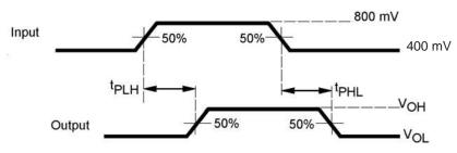
Figure 12. Propagation Delay
