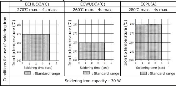
\* Soldering conditions when using soldering iron.
