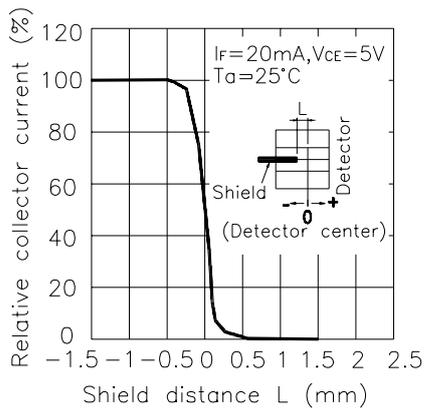
**Fig.7 Relative Collector Current vs. Shield Distance(2)**
