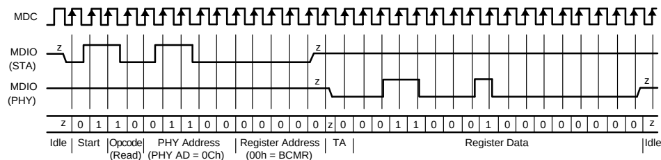
Figure 6-1. Typical MDC/MDIO Read Operation
