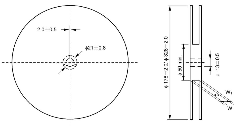
Fig.3 Taping Diagram
