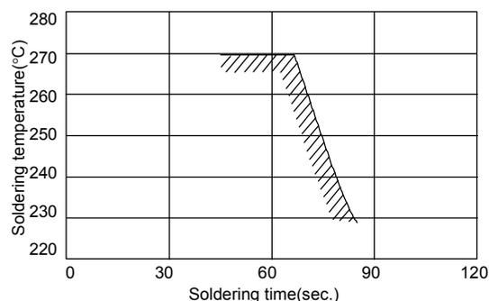
In case of repeated soldering, the accumulated soldering time must be within the range shown above.
