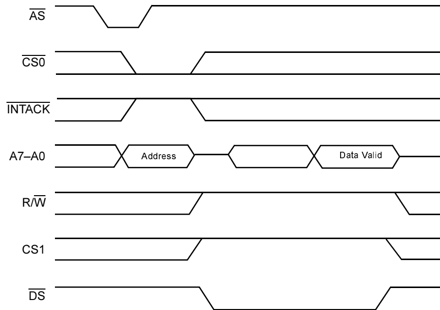
Figure 19. Z80230 Read Cycle Timing
