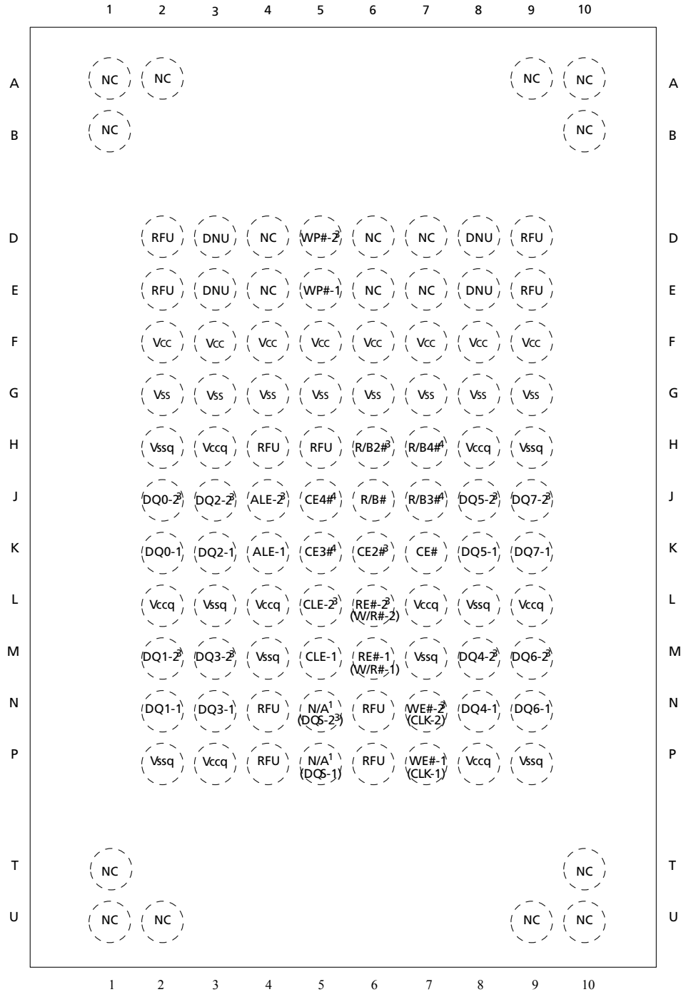
Figure 4: 100-Ball BGA (Ball-Down, Top View)
