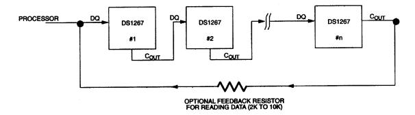
The  $C_{OUT}$  output of the DS1267 can be used to drive the DQ input of another DS1267. When connecting multiple devices, the total number of bits transmitted is always 17 times the number of DS1267s in the daisy chain.
