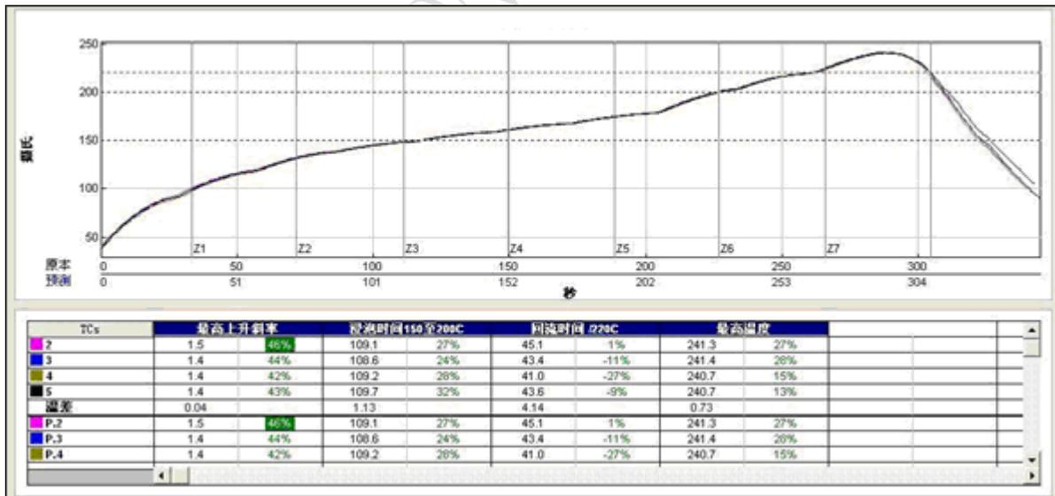
Figure 8: The Ramp-Soak-Spike reflow profile of SIM33ELA
