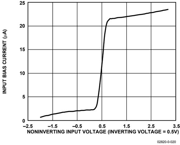
Figure 12. Input Bias Current vs. Input Voltage
