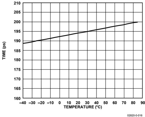
Figure 14. Rise Time vs. Temperature
