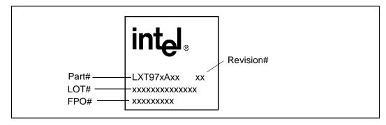
The silicon stepping in the LXT971A/972A Data Sheet is referred to as "Manufacturer's Revision Number." The silicon stepping number may be read by software from Register 3, bits 3:0 in the LXT971A/972A7 transceivers.
