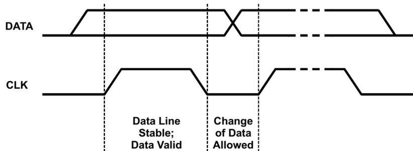
Figure 30. Bit Transfer on the Serial Interface
