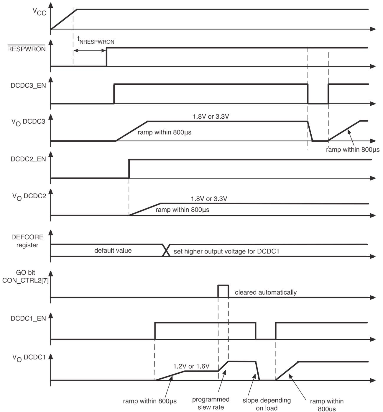
Figure 29. DVS Timing
