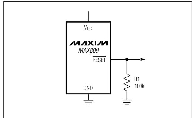
Figure 2.  $\overline{\text{RESET}}$  Valid to  $V_{\text{CC}} = \text{Ground}$  Circuit
