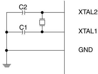
The Oscillator can operate in three different modes, each optimized for a specific frequency range. The operating mode is selected by the fuses CKSEL3..1 as shown in Table 8.
