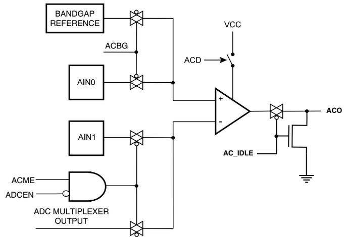
**Figure 129.** General Boundary-scan Cell used for Signals for Comparator and ADC
