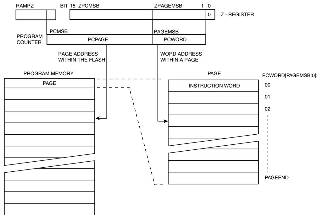
Note: 1. The different variables used in Figure 133 are listed in Table 114 on page 281.
