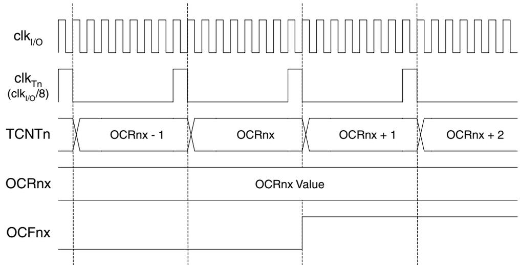
Figure 56 shows the count sequence close to TOP in various modes. When using phase and frequency correct PWM mode the OCRnx Register is updated at BOTTOM. The timing diagrams will be the same, but TOP should be replaced by BOTTOM, TOP-1 by BOTTOM+1 and so on. The same renaming applies for modes that set the TOVn flag at BOTTOM.
