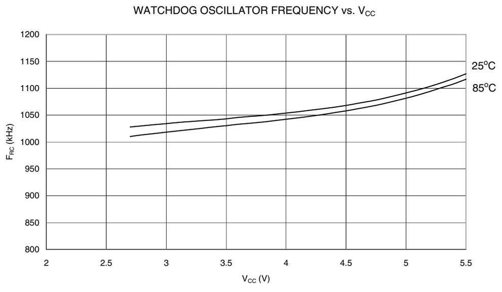
**Figure 195.** RC Oscillator Frequency vs. Temperature (the devices are calibrated to 1 MHz at  $V_{cc} = 5V$ ,  $T=25c$ )
