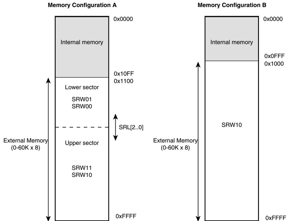
Note: ATmega128 in non ATmega103 compatibility mode: Memory Configuration A is available (Memory Configuration B N/A)
