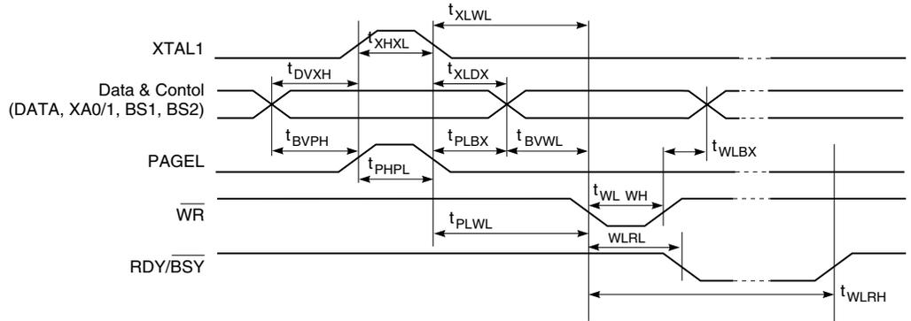
**Figure 141.** Parallel Programming Timing, Loading Sequence with Timing Requirements
