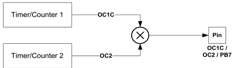
When the modulator is enabled, the two output compare channels are modulated together as shown in the block diagram (Figure 71).
