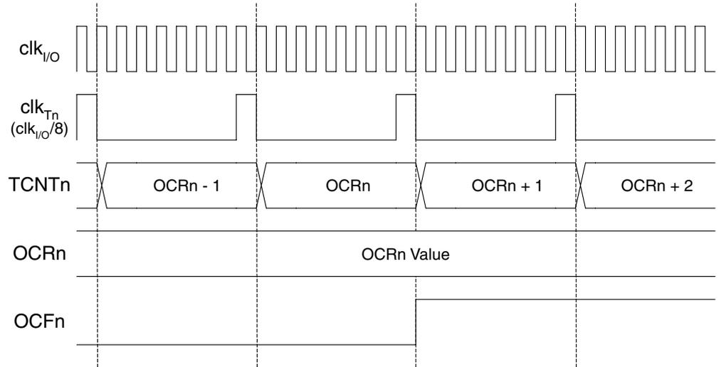
Figure 70 shows the setting of OCF2 and the clearing of TCNT2 in CTC mode.
