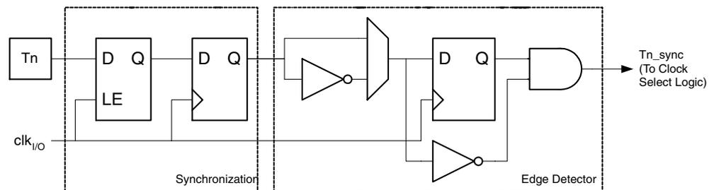
The synchronization and edge detector logic introduces a delay of 2.5 to 3.5 system clock cycles from an edge has been applied to the Tn pin to the counter is updated.
