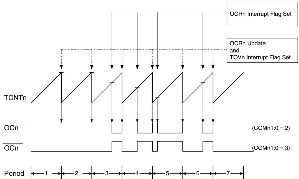
The Timer/Counter overflow flag (TOV2) is set each time the counter reaches Max. If the interrupt is enabled, the interrupt handler routine can be used for updating the compare value.
