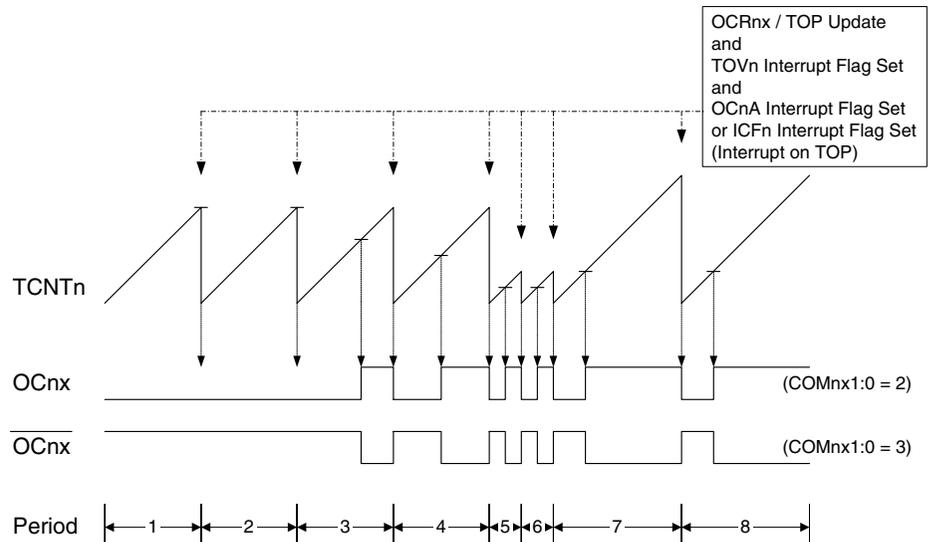
The Timer/Counter Overflow Flag (TOVn) is set each time the counter reaches TOP. In addition the OCnA or ICFn flag is set at the same timer clock cycle as TOVn is set when either OCRnA or ICRn is used for defining the TOP value. If one of the interrupts are enabled, the interrupt handler routine can be used for updating the TOP and compare values.
