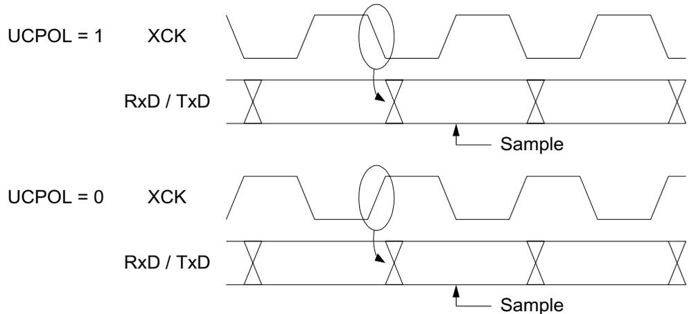
The UCPOL bit UCRSC selects which XCK clock edge is used for data sampling and which is used for data change. As Figure 80 shows, when UCPOL is zero the data will be changed at rising XCK edge and sampled at falling XCK edge. If UCPOL is set, the data will be changed at falling XCK edge and sampled at rising XCK edge.
