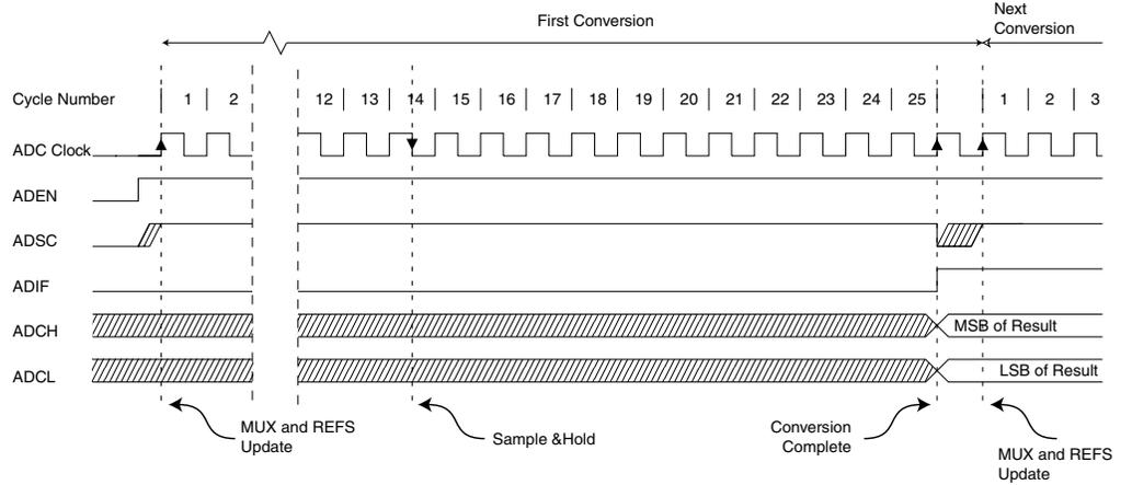
**Figure 110. ADC Timing Diagram, Single Conversion**
