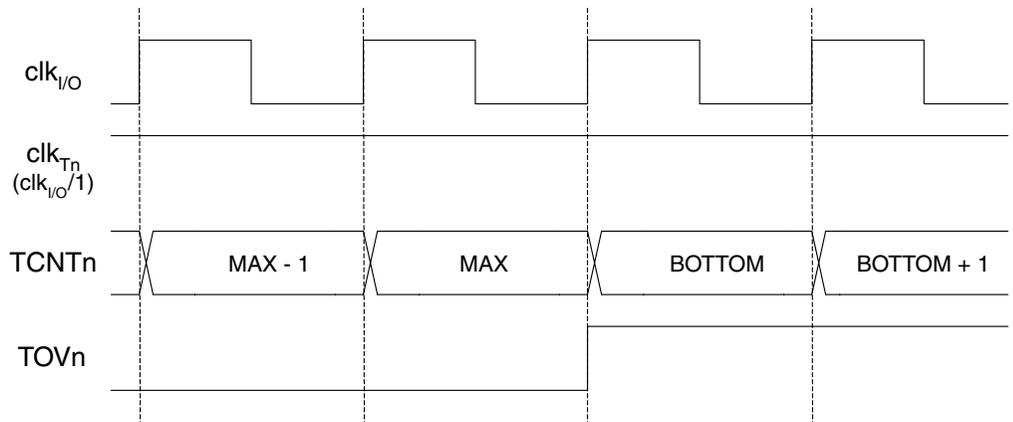
Figure 68 shows the same timing data, but with the prescaler enabled.
