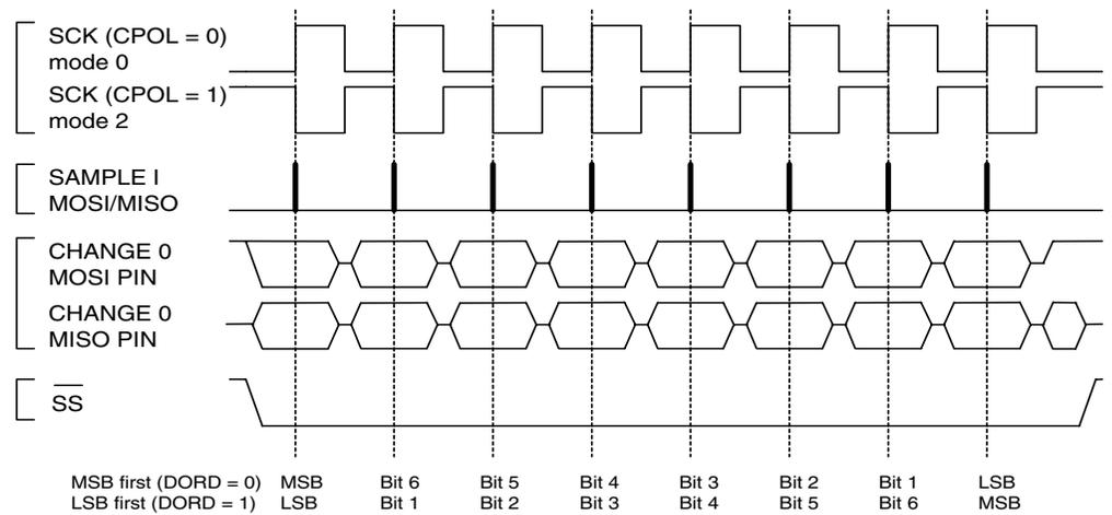
**Figure 77.** SPI Transfer Format with CPHA = 1
