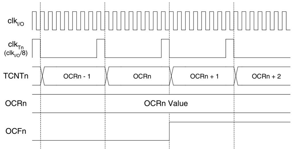
Figure 43 shows the setting of OCF0 and the clearing of TCNT0 in CTC mode.
