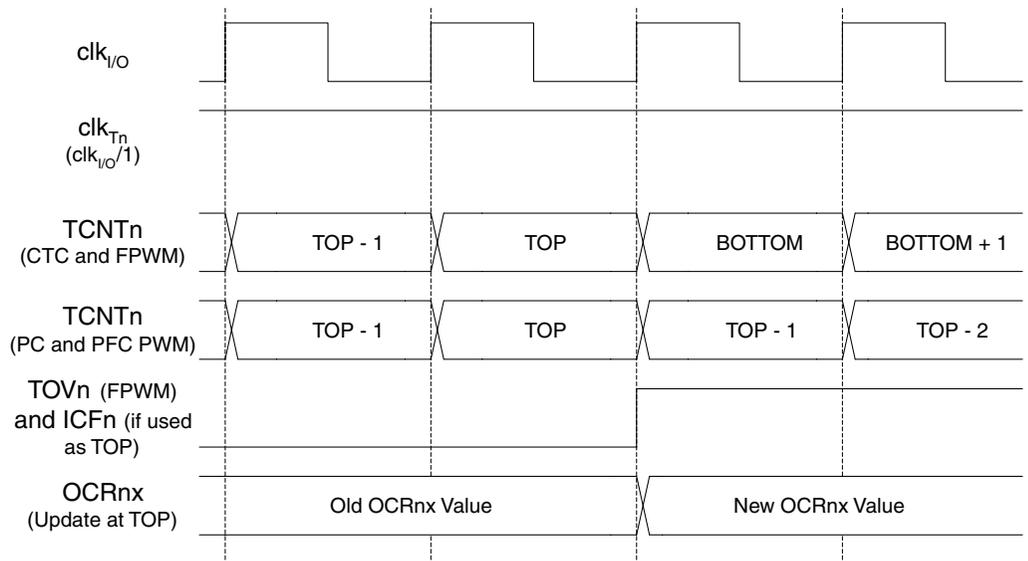
Figure 57 shows the same timing data, but with the prescaler enabled.
