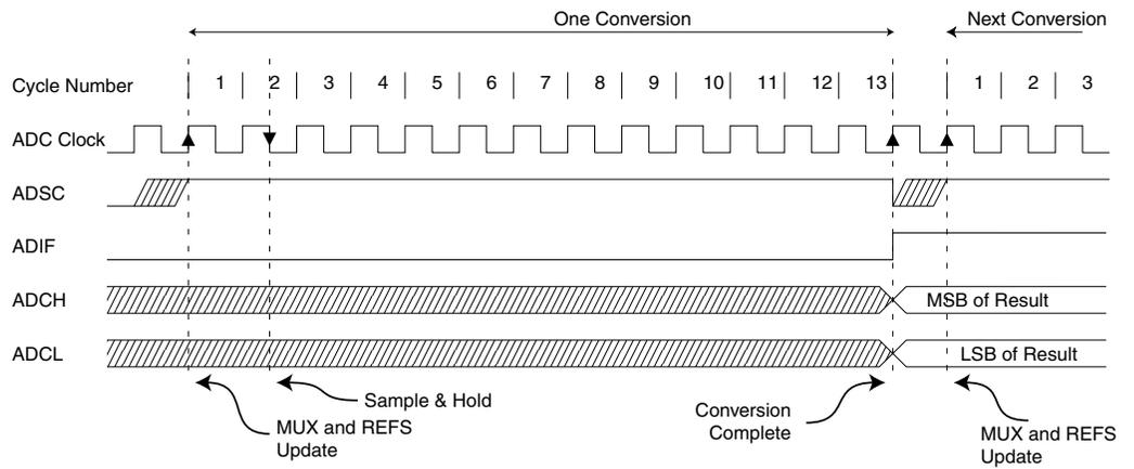
**Figure 111. ADC Timing Diagram, Free Running Conversion**
