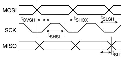
**Table 130.** SPI Serial Programming Characteristics,  $T_A = -40^{\circ}\text{C}$  to  $85^{\circ}\text{C}$ ,  $V_{CC} = 2.7\text{V} - 5.5\text{V}$  (Unless Otherwise Noted)
