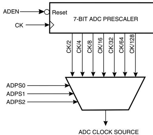
By default, the successive approximation circuitry requires an input clock frequency between 50 kHz and 200 kHz to get maximum resolution. If a lower resolution than 10 bits is needed, the input clock frequency to the ADC can be higher than 200 kHz to get a higher sample rate. Alternatively, setting the ADHSM bit in SFIOR allows an increased ADC clock frequency at the expense of higher power consumption.
