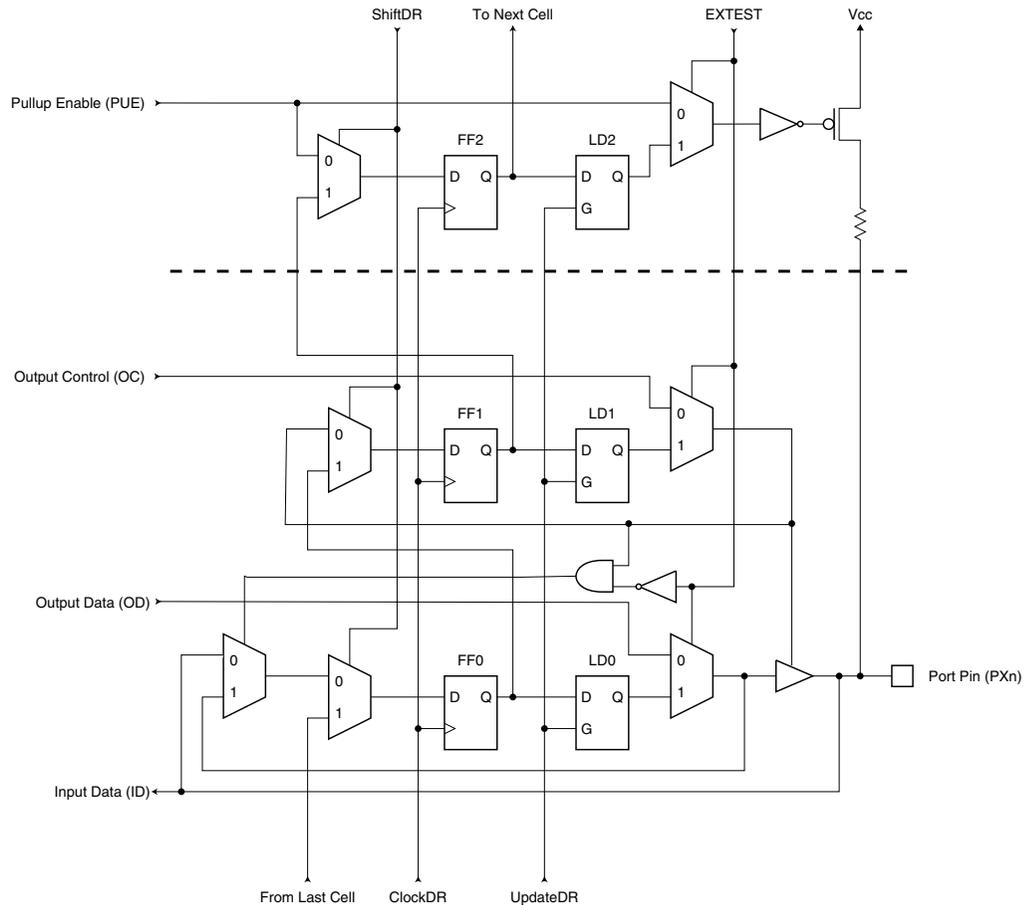
**Figure 124. General Port Pin Schematic diagram**
