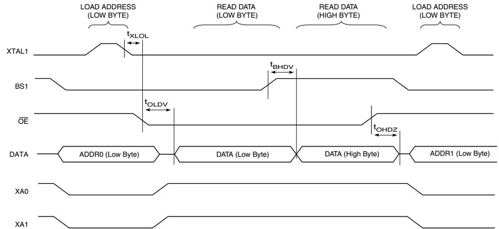
Note: The timing requirements shown in Figure 140 (i.e.  $t_{DVXH}$ ,  $t_{XHXL}$ , and  $t_{XLDX}$ ) also apply to reading operation.
