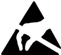
**ESDs** may be destroyed by voltages and energies well below the perception threshold of persons. Voltages of this kind occur as soon as a device or an assembly is touched by a person who is not electrostatically discharged . Devices exposed to such overvoltages cannot immediately be detected as defective in the majority of cases since faulty behavior may occur only after a long period of operation.
