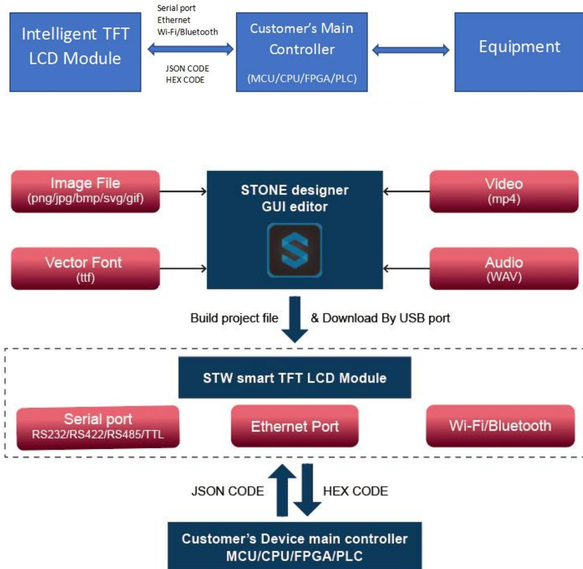
Figure 1.3-1 Configuration and process control phase
