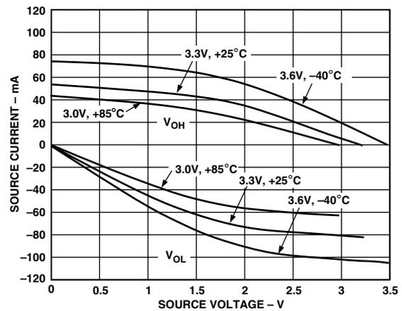
Figure 32. ADSP-21062 Typical Drive Currents ( $V_{DD} = 3.3 V$ )
