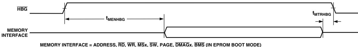
MEMORY INTERFACE = ADDRESS,  $\overline{\text{RD}}$ ,  $\overline{\text{WR}}$ ,  $\overline{\text{MSx}}$ ,  $\overline{\text{SW}}$ , PAGE,  $\overline{\text{DMAGx}}$ ,  $\overline{\text{BMS}}$  (IN EPROM BOOT MODE)
