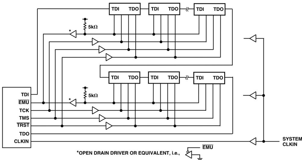
Figure 7. JTAG Clocktree for Multiple ADSP-2106x Systems
