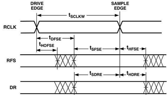
NOTE: EITHER THE RISING EDGE OR FALLING EDGE OF RCLK, TCLK CAN BE USED AS THE ACTIVE SAMPLING EDGE.
