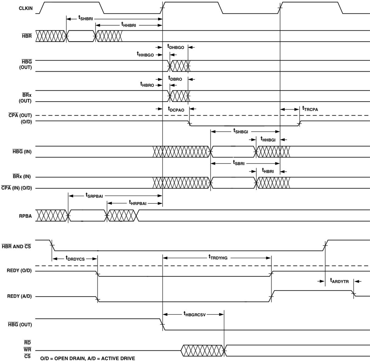
Figure 17. Multiprocessor Bus Request and Host Bus Request
