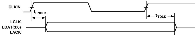
LINK PORT ENABLE OR THREE-STATE TAKES EFFECT TWO CYCLES AFTER A WRITE TO A LINK PORT CONTROL REGISTER.
