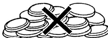
\* Contact between battery poles may form a discharge circuit and lead to heat generation, fire or explosion.
