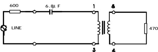
To extend matching and frequency response beyond 30kHz add 4.7nF between pins 1 and 3, and 4.7nF between pins 4 and 6.
