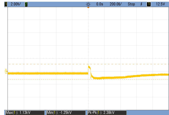
Output voltage waveform (Differential mode 0.90kV)
