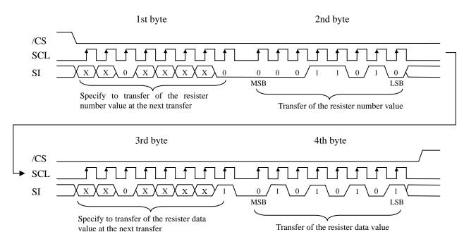
Note1: During 32-bit transfer of the Resister Data, /CS pin (Pin No.35) must be maintained active.
