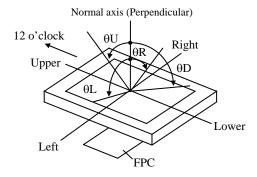
Note4: In reflective mode (Backlight turning OFF), Reflection ratio, Contrast ratio, Chromaticity coordinates and Color gamut are measured as follows.
