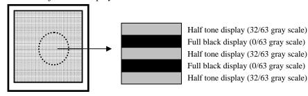
Note2: PPCLK= 5.0MHz, PPHSYNC= 19.53kHz, PPVSYNC= 60Hz, Checkered flag pattern (by EIAJ ED-2522)
