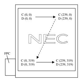
Note1: Meaning of C (X, Y) and D (X, Y)
