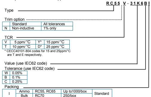
For CECC released product state on order the CECC number and style. Example: RC55Y-31K6BI CECC40101-004 J For SnPb finish instead of Pb-free replace the packing suffix with PB. Example: RC55V-31K6BPB
