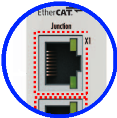
Fig. 12: Identification of FHC port at EK1122-0080 and EK1101-0080
