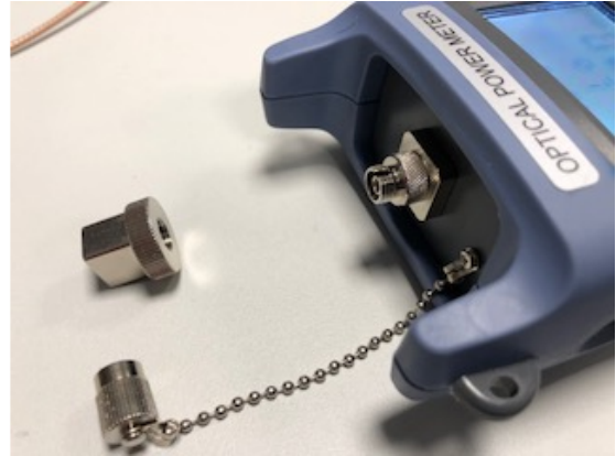
OPM with FC adapter screwed on
