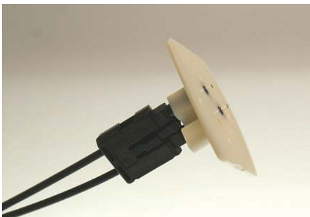
Fig. 57: Sanding gauge with protruding fiber ends
